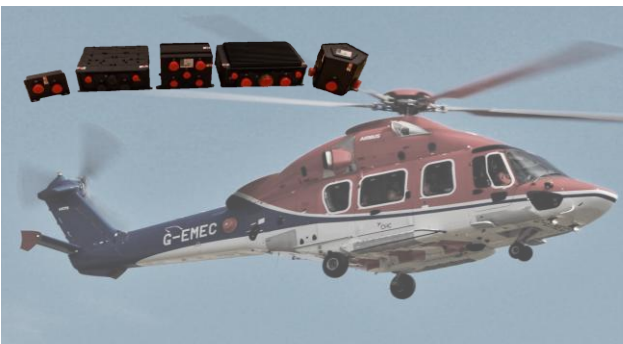
H175 - Ice Detection & De-icing Control System
